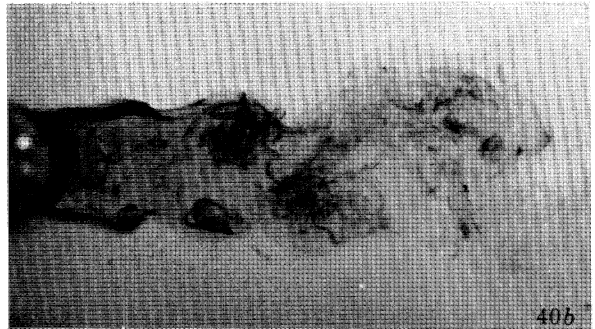
FIGURE 40. Transition waves at Re = 1083 .
