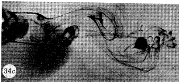
FIGURE 34. The wake of a circular cylinder at Re = 334 . Consecutive views at separation 0.22 period of oscillation.
