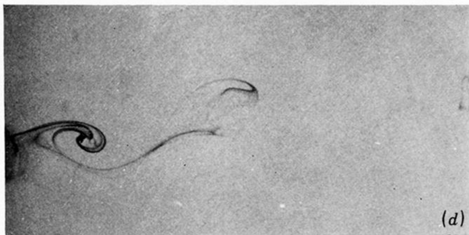
FIGURE 17. The appearance of a knot from above. Wake of a flat plate with a 2% step in its width. Re above and below the step 73.1 and 71.7. Dye on one side of the cylinder only. (a) Wake appearance with no knot present; (b), (c) and (d) Consecutive photographs showing the vortext core linking with the next vortex of the same sign.
