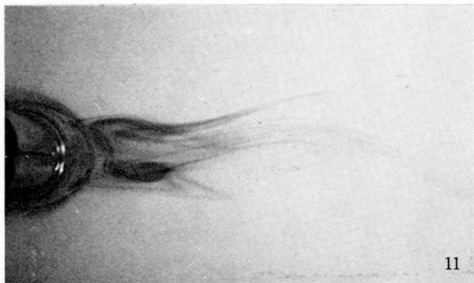
FIGURE 6. Wake of a circular cylinder at Re = 37.8 .
