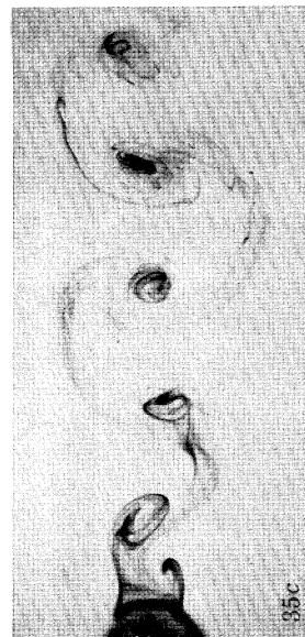
FIGURE 35. The wake of a circular cylinder at Re = 340 . Consecutive views separated by 0.41 period.
