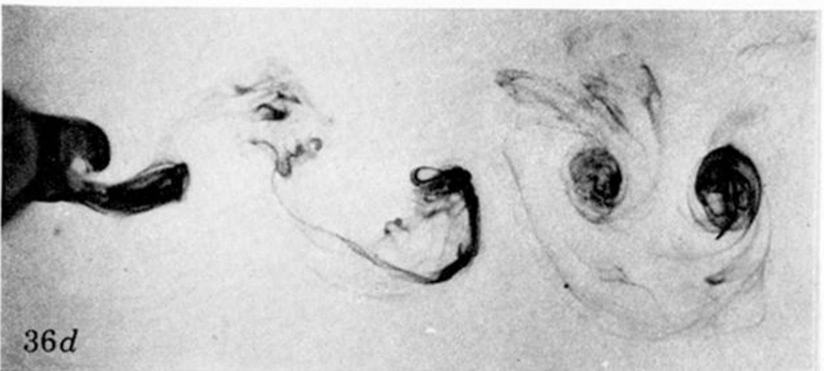
FIGURE 36. The wake of a circular cylinder at Re = 407 . Consecutive views separated by 0.55 period.
