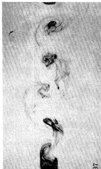
FIGURE 37. The wake of a circular cylinder at Re = 464 .
