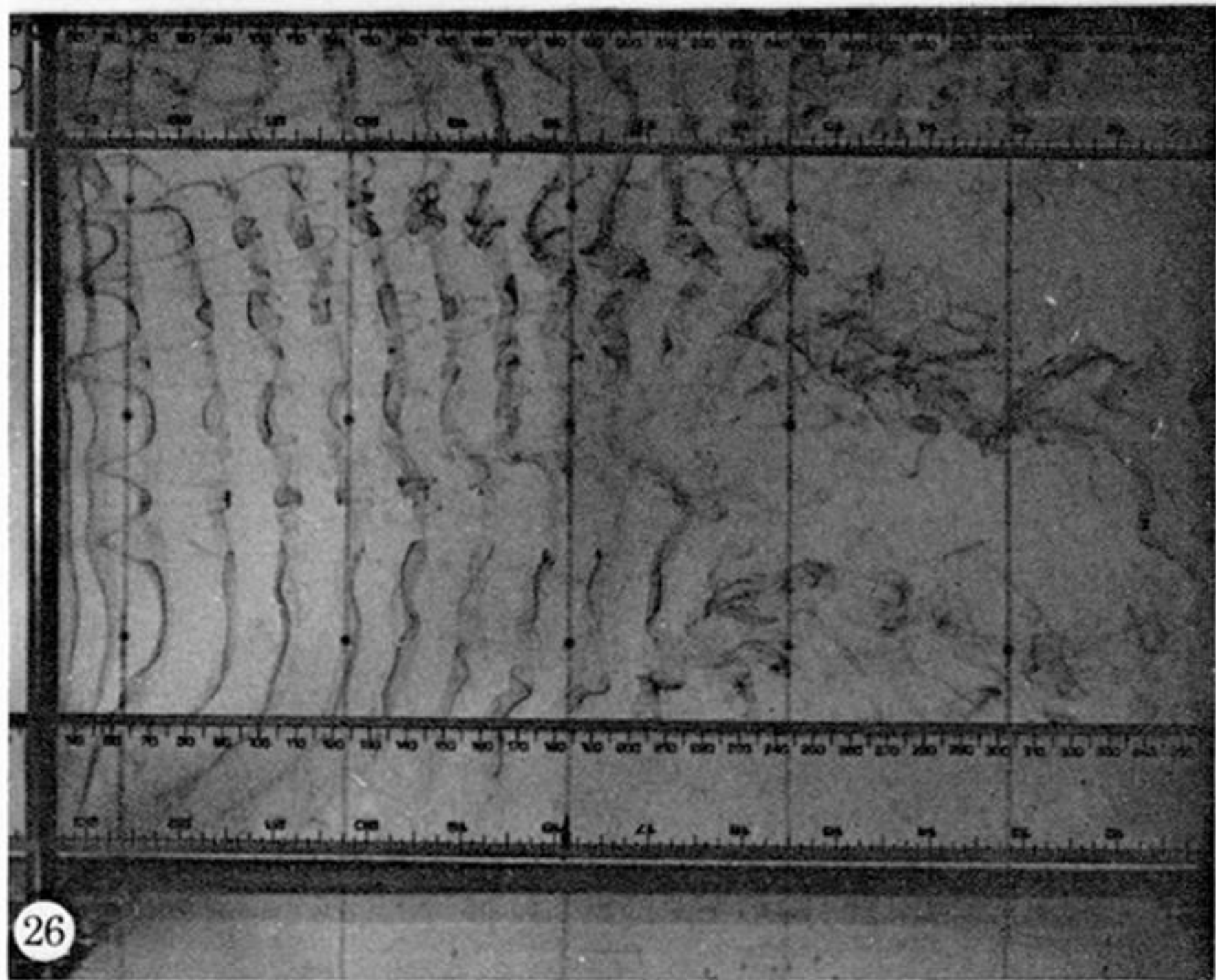
FIGURE 26. Side view of the wake of a circular cylinder at Re = 217 .
