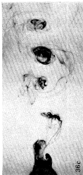
FIGURE 37. The wake of a circular cylinder at Re = 464 .
