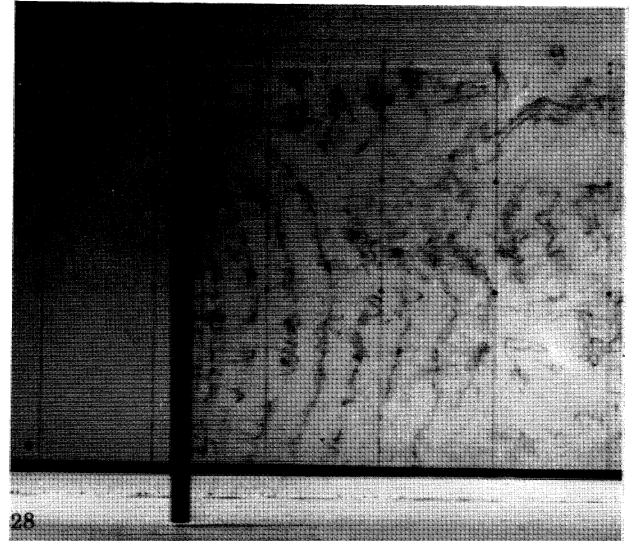
FIGURE 28. Side view of the wake of a circular cylinder at Re = 344 .
